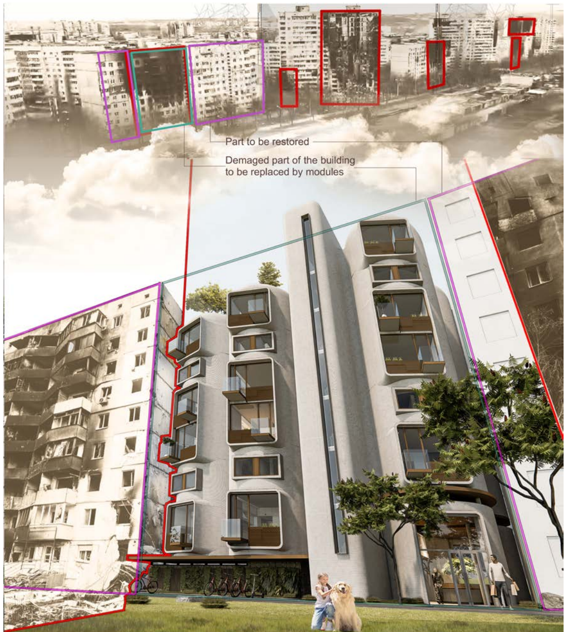
Fig. 6 The vision for 3D-printed infill rebuilding at North Saltivka, Kharkiv, by the architect Kostiantyn Rusiev. Image used by permission of RP Project.
